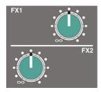
There are two FX sends on the Stereo channels and they take a summed Mono signal of your Stereo Input source. By default the signal is sourced post Fader.
